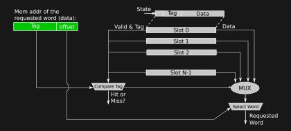
For each data access, all tags of all slots have to be read out to compare with the tag of the requested data's tag.
