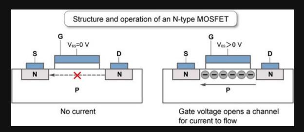
A N-Type MOSFET as an ON/OFF Switch
